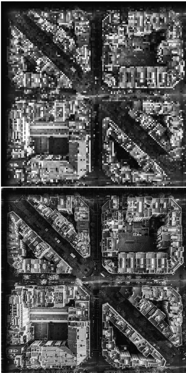
Fig. 6. (Top) The top-left quadrant, sized 128^2 , of the instrument image from an extended scene. (Bottom) The top-left quadrant, sized 2048^2 , in which the truth image was used to model the magnitude for the reconstruction. (Image used with permission, courtesy of Márton Mogorósy photography.)
